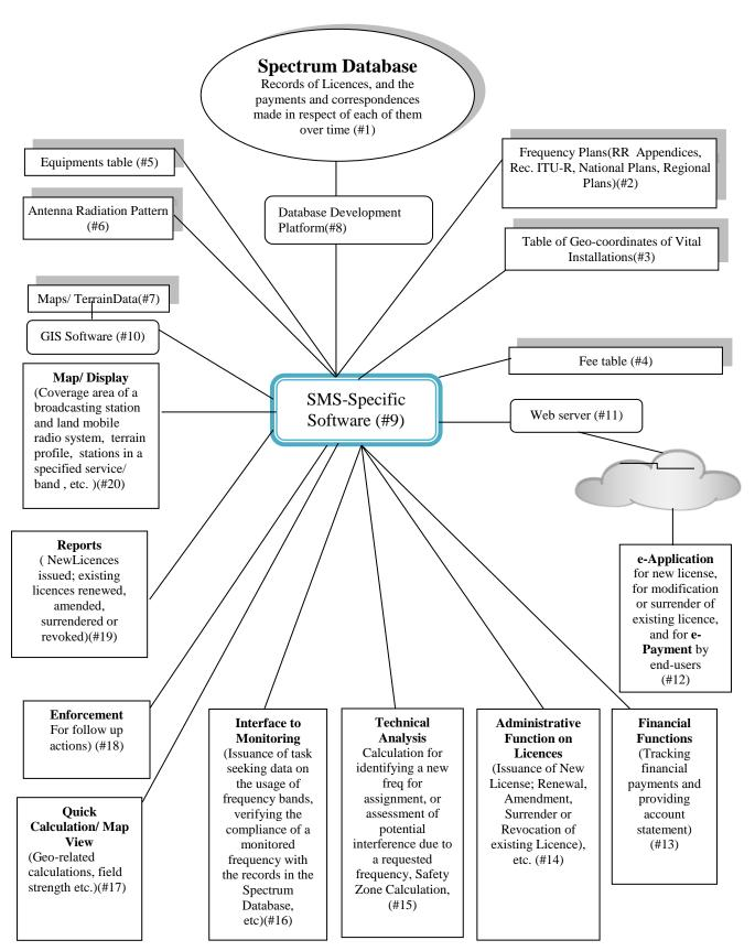
Figure A1. A High Level View of the Architecture of the Spectrum Management System
